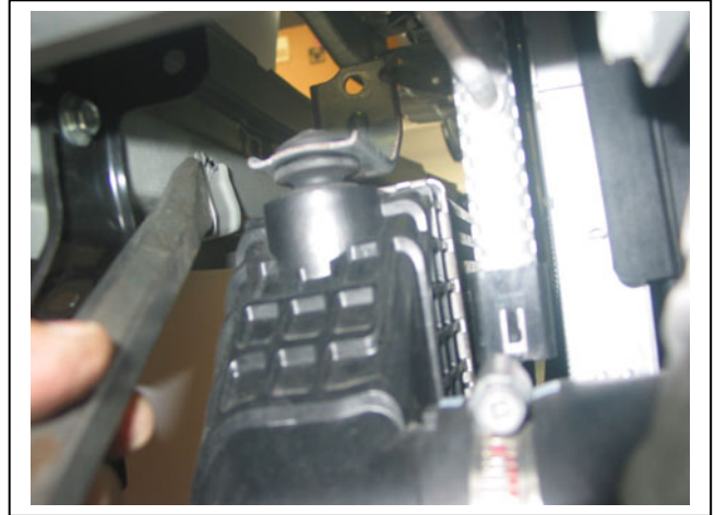
Figure 4: Chisel off temp sensor mount
