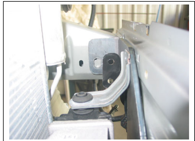
Figure 6: Flattened tab on top intercooler mount
