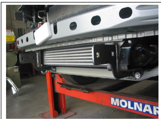
Figure 7: ECB steel mounting brackets fitted.
