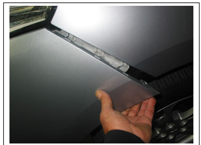
Figure 2: Carefully remove bumper from guard clips
