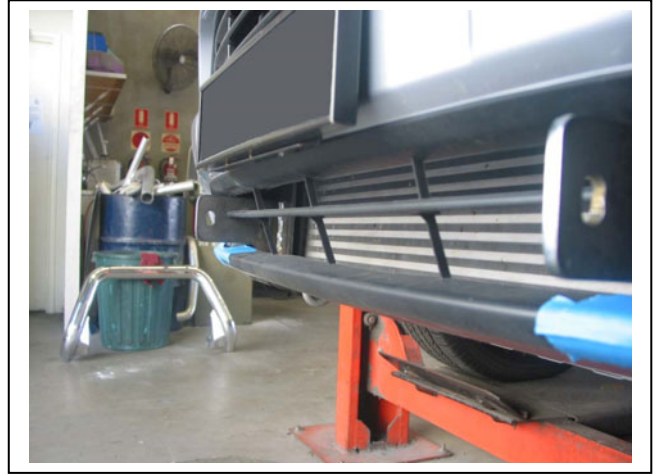
Figure 10: ECB steel mounting brackets with bumper fitted.
